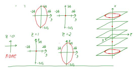
Need way to connect" layers  $\Rightarrow$  use w=y, and view trace when y=0:  $\chi^2-\frac{z^2}{q}=|+\frac{Q^2}{q}|$  which means layers connected by a hyperbola. Surface: hyperboloid of 2 sheets.
